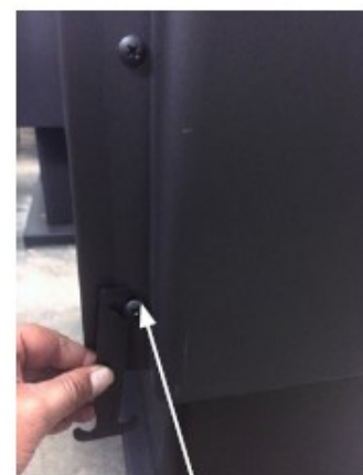
Loosen screw and insert storage bracket
