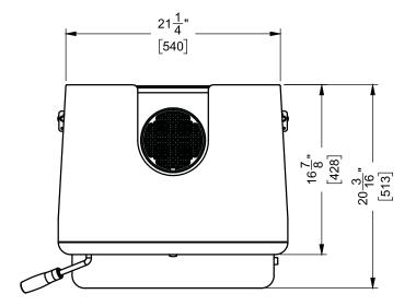
6" (152mm) Diameter STANDARD FLUE ADAPTOR
