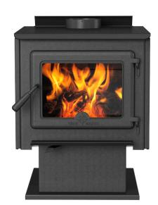
**NEW FOR 2015.** The TN20 features entry-level tubes as part of the combustion system, offering a cost effective solution for the price-minded wood burner. Constructed with standard 10-guage steel, the TN20 features a gasketed cast iron door, clean glass airwash, and high efficiency. Available with legs or a pedestal base, the TN20 offers an exceptional cost – performance ratio.
